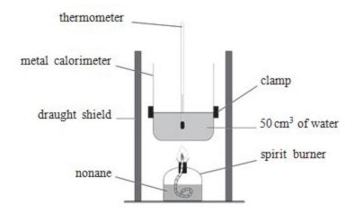
(i) Iwan measured the mass of the spirit burner at the start and end of the experiment and found that 0.20 g of nonane had been burned. Calculate the number of moles of nonane present in 0.20 g.
